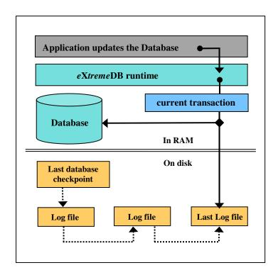
Logging may be set to different levels of transaction durability. Cleanup of outdated logs and database images ("checkpoints") can be synchronized with checkpoint completion, or delegated to a background task. To provide the greatest flexibility, McObject provides a rich array of transaction logging control parameters, including depth of the recovery tree and maximum transaction log file size.
